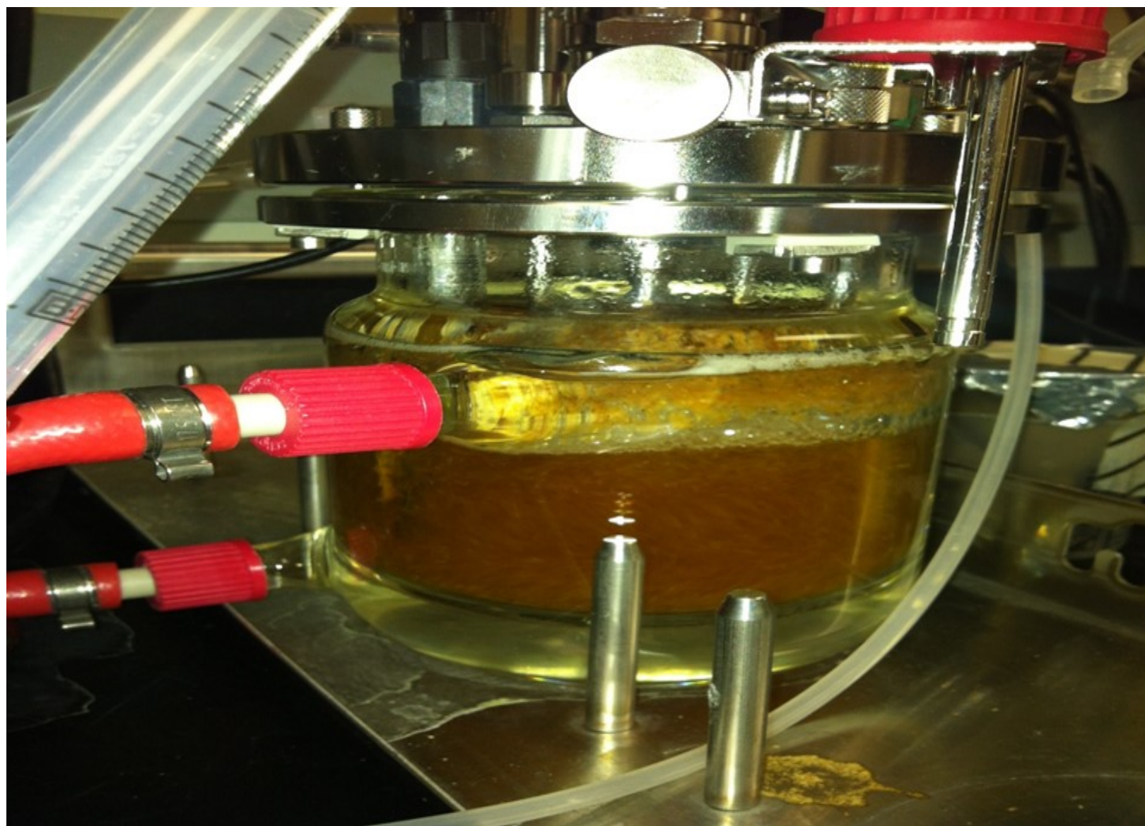
Fig.4 Bacteria convert corn stover to hydrogen in a fermentation reactor at the National Renewable Energy Laboratory. Photo by Sarah Studer, DOE
