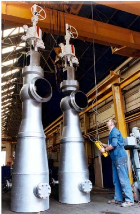
Figure 1-WEIR Turbine Bypass Valve
