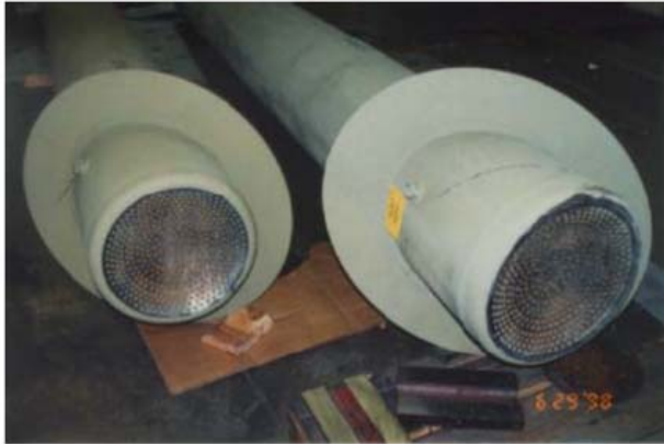
Figure 4-Spargers Designed to Spray Out the End to Eliminate Steam Impinging Upon the Condenser Tubes
