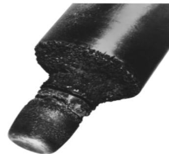
Fig. 7 Effect of Cavitation on the valve trim
